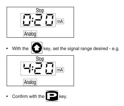
• For the 0 mA signal you receive the display of the stroking rate 0 strokes per minute and the error message "Error" with "Analog" flashing, as the control signal is below 4 mA.
