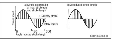
Set stroke length dependent on the required delivery capacity.
