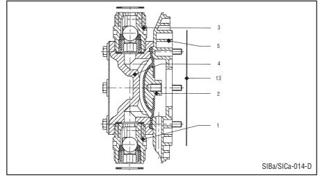
The tightening torques of the liquid end screws should be checked every 3 months for the PVT material version.
