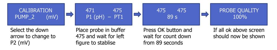
Probe quality will be shown in 100%, 75%, 50%, 25%. If "CALIBRATION ERROR" is displayed probe must be replaced. If 25% or 50% is shown replacement probe should be considered as soon as possible
