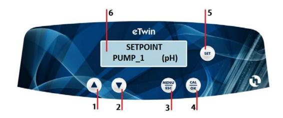
With the pump running hold down button 5 (SET) for around 5 seconds. This will take you into setpoint menu. Up and down arrows will change between pumps 1 and 2.
