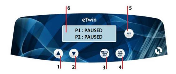
Whilst in PAUSED mode holding down button 1 will prime P1 (pump number 1) and holding down Button 2 will prime P2 (pump number 2) Pump will stop priming when either of the buttons are released
