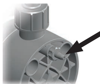
Fig. 14: Dosing head venting facility with hose connection
