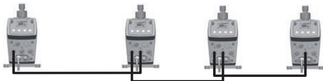
Fig. 17: Synchronization of several dosing pumps by means of stroke feedback and pulse control
